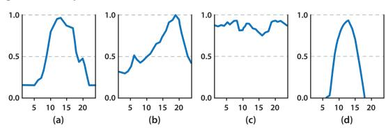
Note: Load profiles are shown for (a) commercial, (b) residential, and (c) industrial customers. Figure 7.1d shows an ideal generation profile for a PV facility. All values are expressed as a fraction of annual maximum load (or generation in the case of Figure 7d). In each graph, hours of the day are shown on the horizontal axis.
