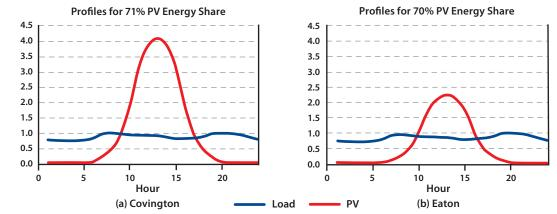
Note: The two graphs contrast a location with low (a) and high (b) insolation. The values in the profiles are expressed as fractions of the peak load of each location.
