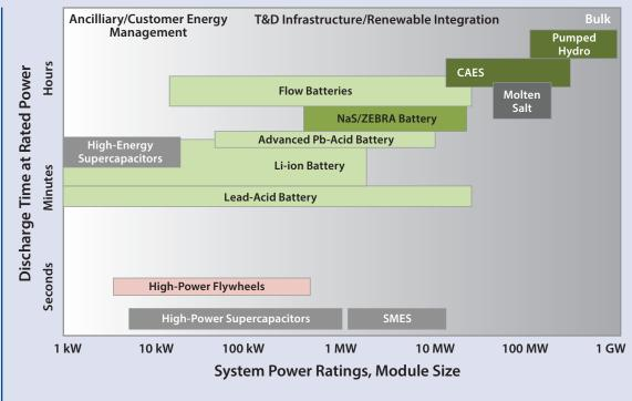
Figure C.2 ESS Technologies and Associated Applications
