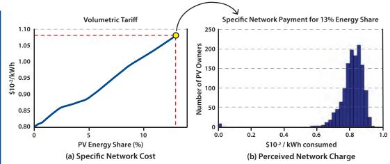
Figure 7.13 Effect of Volumetric Tariff under Net-Metering for the Des Moines Host Network
