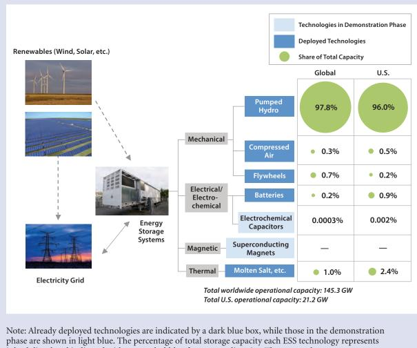
Figure C.1 Grid-Related Energy Storage Technologies Deployed or in the Demonstration Phase<sup>ii</sup>
