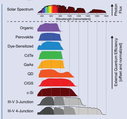
Note: The top part of the figure shows solar photon flux at the earth's surface as a function of wavelength. The types of solar cell technologies included in the bottom part of the figure are described in more detail in Chapter 2.
