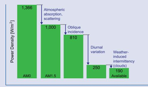
Figure A.1 Reduction in Average Solar Power Density from Different Factors<sup>10,16,18,19</sup>
