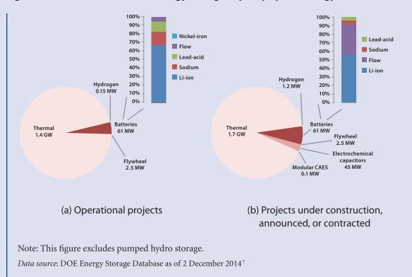
Figure C.3 Global Solar-Related Energy Storage Capacity by Technology
