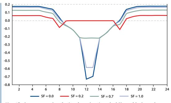
Figure 7.11 Modification of Net Load for Different Energy Storage Factors (SF)
