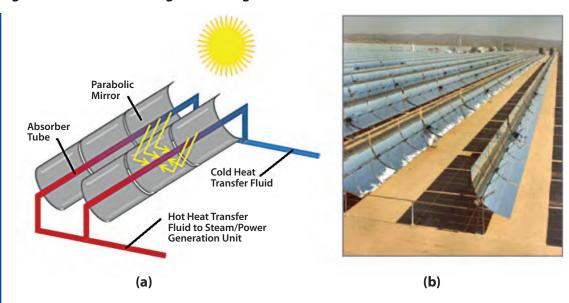
Figure 3.3 Parabolic Trough CSP Design
