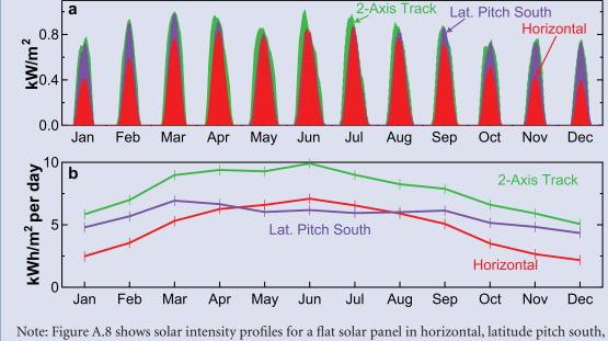
Figure A.8 Daily Irradiance and Monthly Insolation Profiles for Different Solar Panel Arrangements
