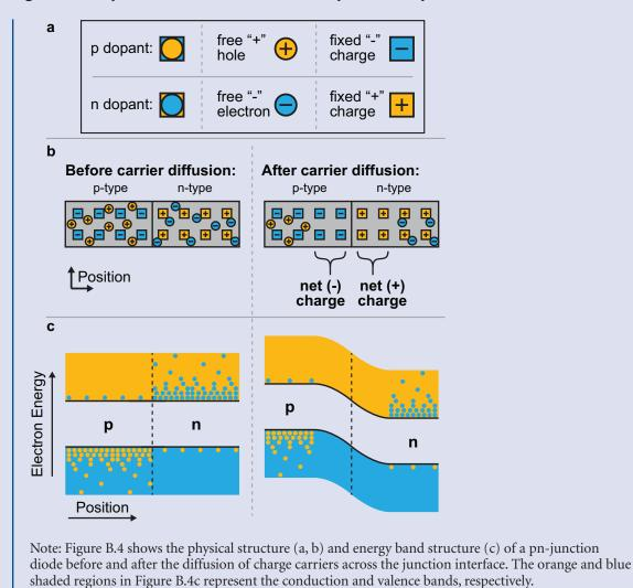
Figure B.4 Physical Structure and Electric Properties of a pn-Junction Diode
