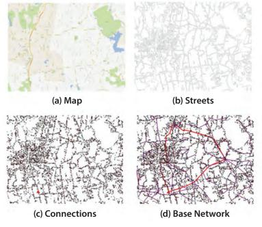
Note: The initial map of the region under study is shown in (a), while (b) and (c) illustrate the assignment of network users to geographic locations and (c) shows the network designed by RNM with three voltage levels — LV in green, MV in magenta, and HV in red.
