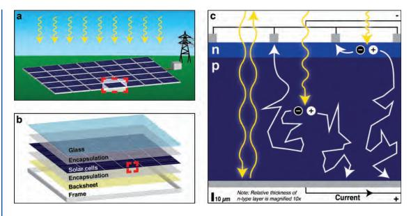
(a) Illustration of grid-connected PV system
