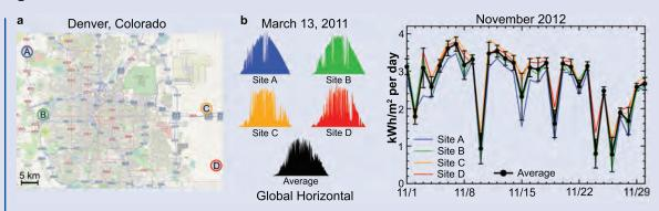
Note: Figure A.7 shows irradiance profiles for four separate measurement sites in the Denver area, including (a) a map showing the location of the measurement sites;<sup>20</sup> (b) the global horizontal irradiance profile at each of the sites and the four-site average on March 13, 2011, a day with many minute-to-minute variations; and (c) daily average insolation for each site and for the four-site average over the month of November 2012, a month with many day-to-day variations.<sup>17</sup>
