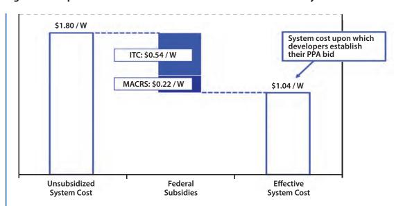
Figure 4.9 Impact of Federal Subsidies on the Effective Cost of Utility-Scale PV
