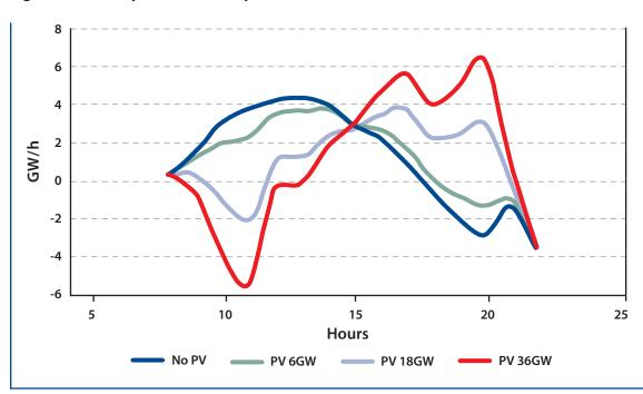
Figure 8.3 Hourly Net Load Ramps for Different Levels of Solar PV Penetration
