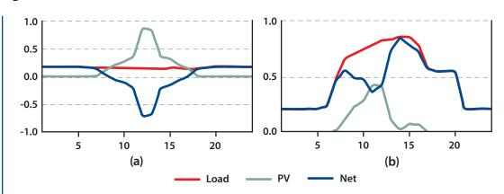
Note: The graphs shown are for a commercial customer in the city of Lancaster, California. All the values are expressed as a fraction of the annual maximum load. Hours of the day are on the horizontal axis.
