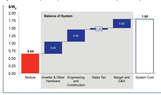
Figure 4.7 Stair Step Build-Up of Estimated Costs for a Utility-Scale PV System
