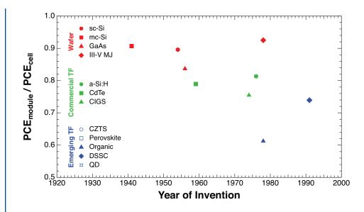
Figure 10.5 Effect of Development Time on Record Efficiencies of Solar Cells and Modules
