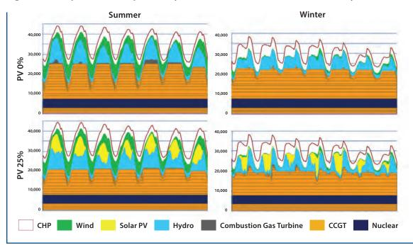
Figure 8.12 Operational Impact of Hydro Resources in the California-Like System
