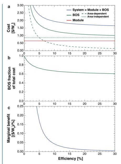
Figure 10.4 Effect of Module Efficiency on the Cost of a Crystalline Silicon PV System
