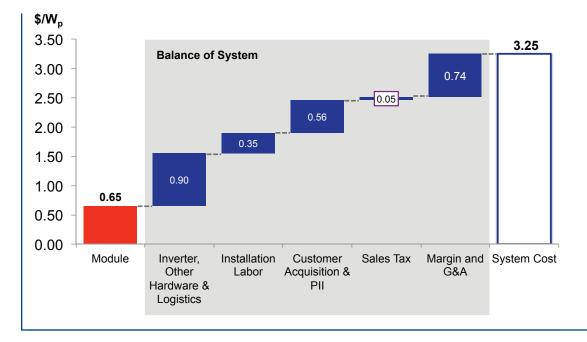
Figure 4.8 Stair Step Build-Up of Estimated Costs for a Residential PV System<sup>v</sup>
