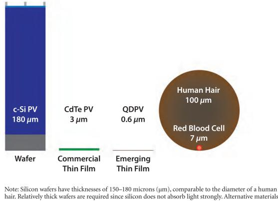
Figure 2.4 Solar Cell Thickness by Technology Classification
