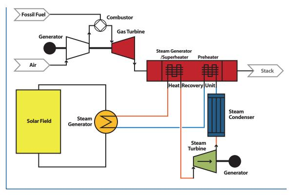
Figure 3.11 Integrated Solar Combined Cycle System
