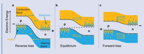
Note: The energy bands shown in Figure B.5 correspond to reverse bias (a), equilibrium (b), and forward bias (c) conditions. Blue and orange arrows represent electron flux and hole flux, respectively.
