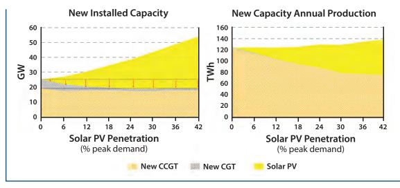
Figure 8.15 Capacity Value of Solar PV in the ERCOT and California Systems
